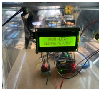
Figure 12. Roof Status Display is Closing
