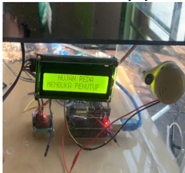
Figure 13. Roof Status Display While Opening
