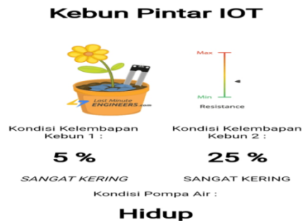
Figure 7. Results of dry soil testing on a mobile phone
